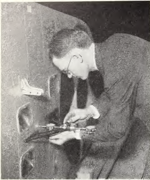
Cellulose acetate butyrate dope for fabric-covered wing and control surfaces on aircraft was developed by the National Bureau of Standards to replace the highly flammable and less durable cellulose nitrate dope. The dope developed by this Bureau was used on Navy carrier-based aircraft during World War II and has also been used extensively on light civilian airplanes. The photograph shows a tautness reading being made on a doped fabric surface of an airplane wing.
